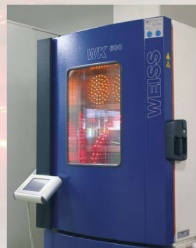
In-house climate testing of the boards
